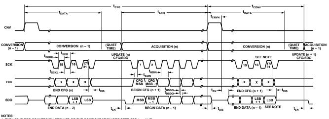
I. THE LSB IS FOR CONVERSION RESULTS OR THE CONFIGURATION REGISTER CFG (n – 1) IF 16 SCK FALLING EDGES = LSB OF CONVERSION RESULTS.
