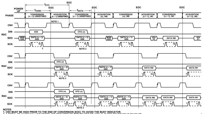
CNV MUST BE HIGH PRIOR TO THE END OF CONVERSION (EOC) TO AVOID THE BUSY INDICATOR. A TOTAL OF 16 SCK FALLING EDGES ARE REQUIRED TO RETURN SDO TO HIGH-Z. IF CFG READBACK IS ENABLED, A TOTAL OF 30 SCK FALLING EDGES IS REQUIRED TO RETURN SDO TO HIGH-Z.
