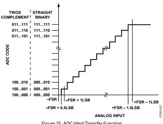
Figure 25. ADC Ideal Transfer Function
