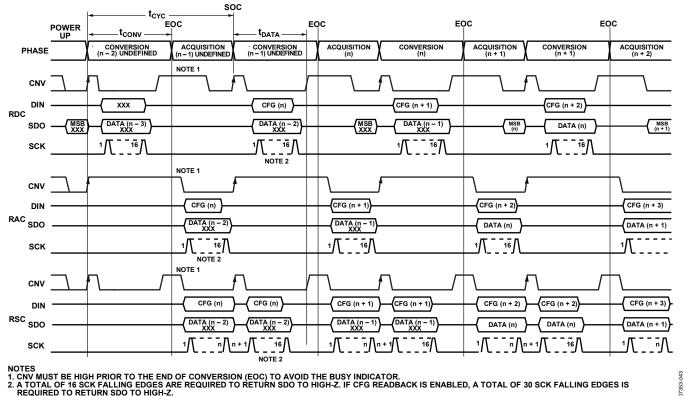
A TOTAL OF 16 SCK FALLING EDGES ARE REQUIRED TO RETURN SDO TO HIGH-Z. IF CFG READBACK IS ENABLED, A TOTAL OF 30 SCK FALLING EDGES IS REQUIRED TO RETURN SDO TO HIGH-Z.
