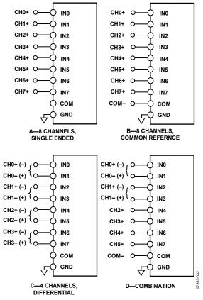
Figure 30. Multiplexed Analog Input Configurations
