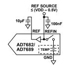
Figure 32. External Reference Using Internal Buffer
