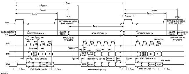
NOTES 1. THE LSB 15 SCK F SB IS FOR CONVERSION RESULTS OR THE CONFIGURATION REGISTER CFG (n – 1) IF K FALLING EDGES = LSB OF CONVERSION RESULTS. K FALLING EDGES = LSB OF CONFIGURATION REGISTER. HE 16TH OR 30TH SCK FALLING EDGE, SDO IS DRIVEN TO HIGH IMPENDANCE.
