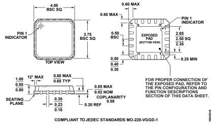
Figure 44. 20-Lead Lead Frame Chip Scale Package (LFCSP\_VQ) 4 mm × 4 mm Body, Very Thin Quad (CP-20-4) Dimensions shown in millimeters
