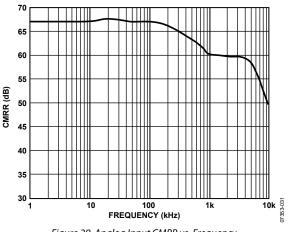
Figure 29. Analog Input CMRR vs. Frequency
